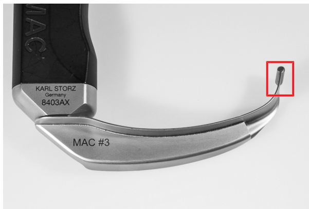
Defect pattern: Blade tip bent
